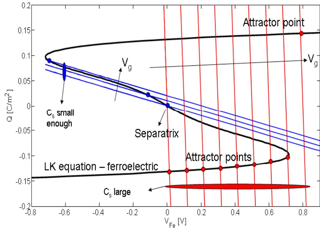
The Negative Capacitance (NC) region is unstable, but it could be accessed if the semiconductor capacitance ( $C_s$ ) is small with regard to the ferroelectric capacitance ( $C_{fe}$ )
