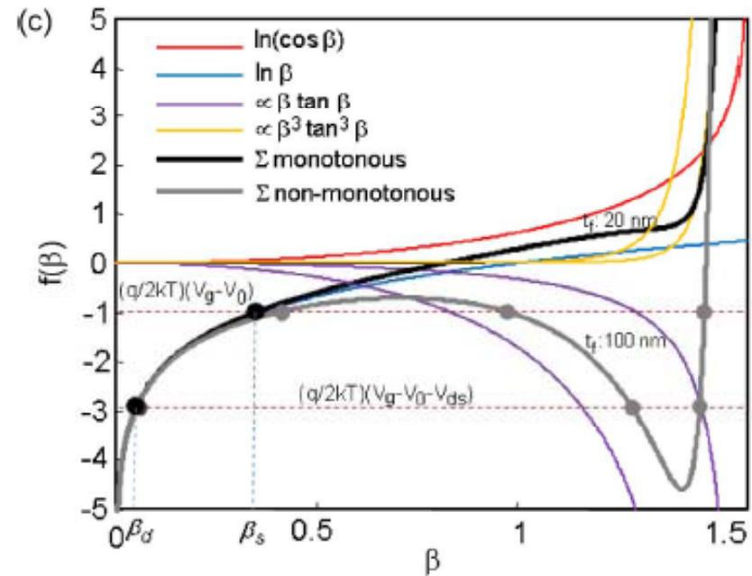
Determination of  $\beta$  can be geometrically interpreted as the intersection of  $f(\beta)$  with the load line  $(q/2kT)(V_g - \Delta\varphi - V)$
